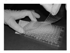
single well cover with a scalpel. The sheet can be quickly spotted manually for hanging drop with an eight-channel pipette or can be incorporated into a robotic system.
